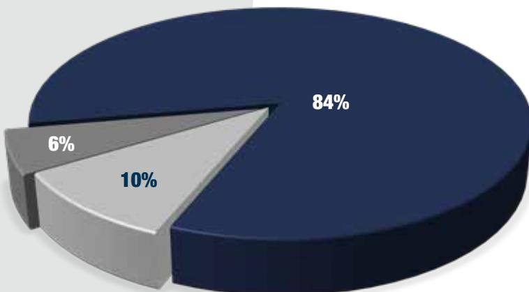
The graph represents the life-cycle cost breakdown of a 37 kW fixed-speed compressor over 5 years of use, assuming 4000 operating hours per year and an energy cost of approximately 0.17 €/kWh.
